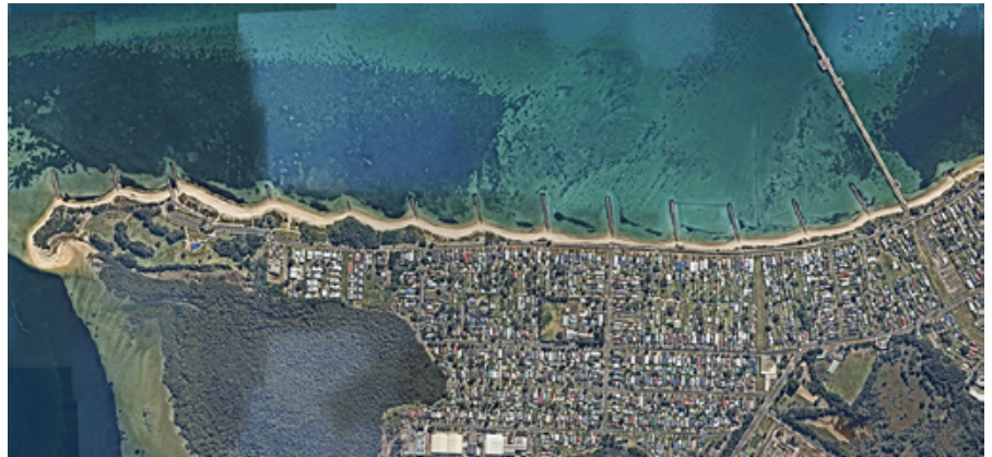
Example of a groyne system at Silver Beach in Kurnell NSW. Source: Nearmap
